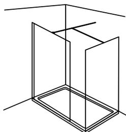
Two wetroom panels can simply combined to create a minimalist walk in design (left) using a joining piece..
